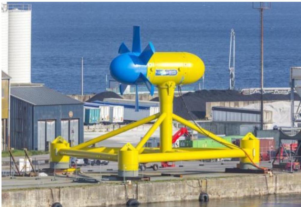
Figure 2.27 Sabella D10 tidal turbine in the Brest assembly area (Paboeuf et al., 2016).
