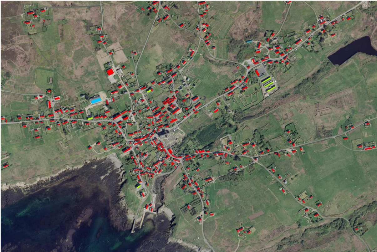
Figure 2.15 Map of Lampaul showing solar rooftop sites. The operating solar PV installation on the sports centre (blue), the planned solar projects (green) and potential rooftop sites (red) are shown. (Base map source: IGN)
