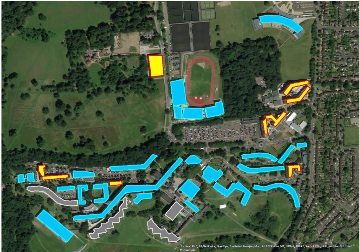
Figure 3.7 GIS of the UEA campus showing buildings with existing solar installations (yellow), buildings with the potential for solar installations (blue) and listed buildings (grey).
