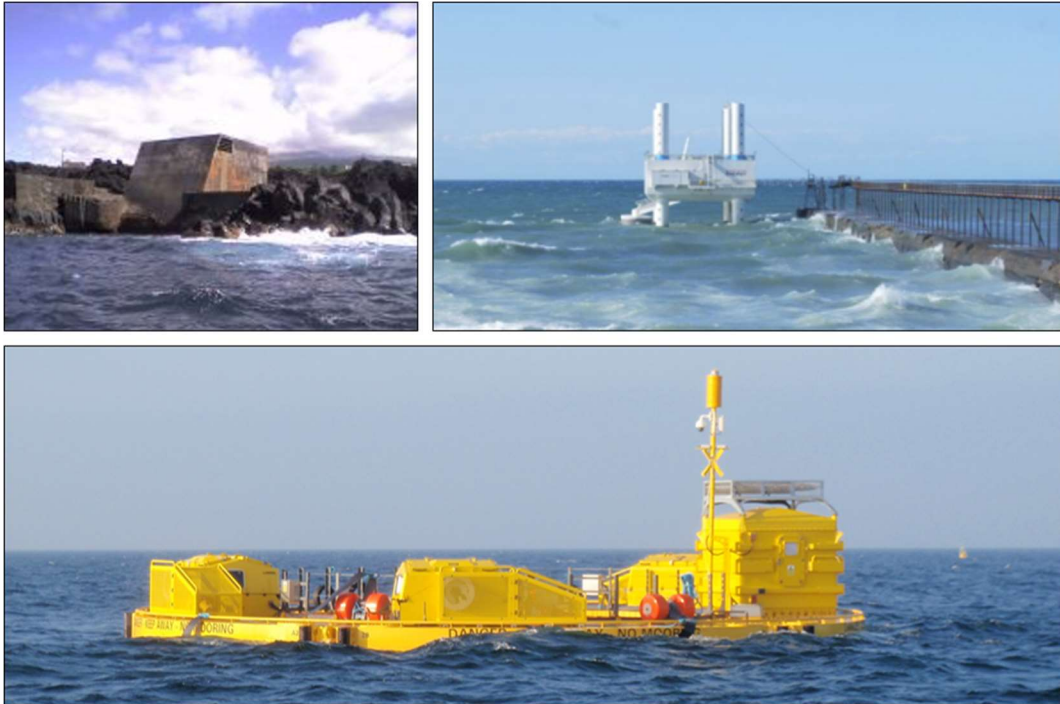
Figure 3-4: Examples of wave energy devices: the onshore Pico Plant OWC in the Azores (source: Pico OWC, 2006) (top left); the nearshore Wavestar device with point absorber floats (source: Wavestar, n.d.) (top right); the offshore Fred Olsen 'BOLT II Lifesaver' (bottom).
