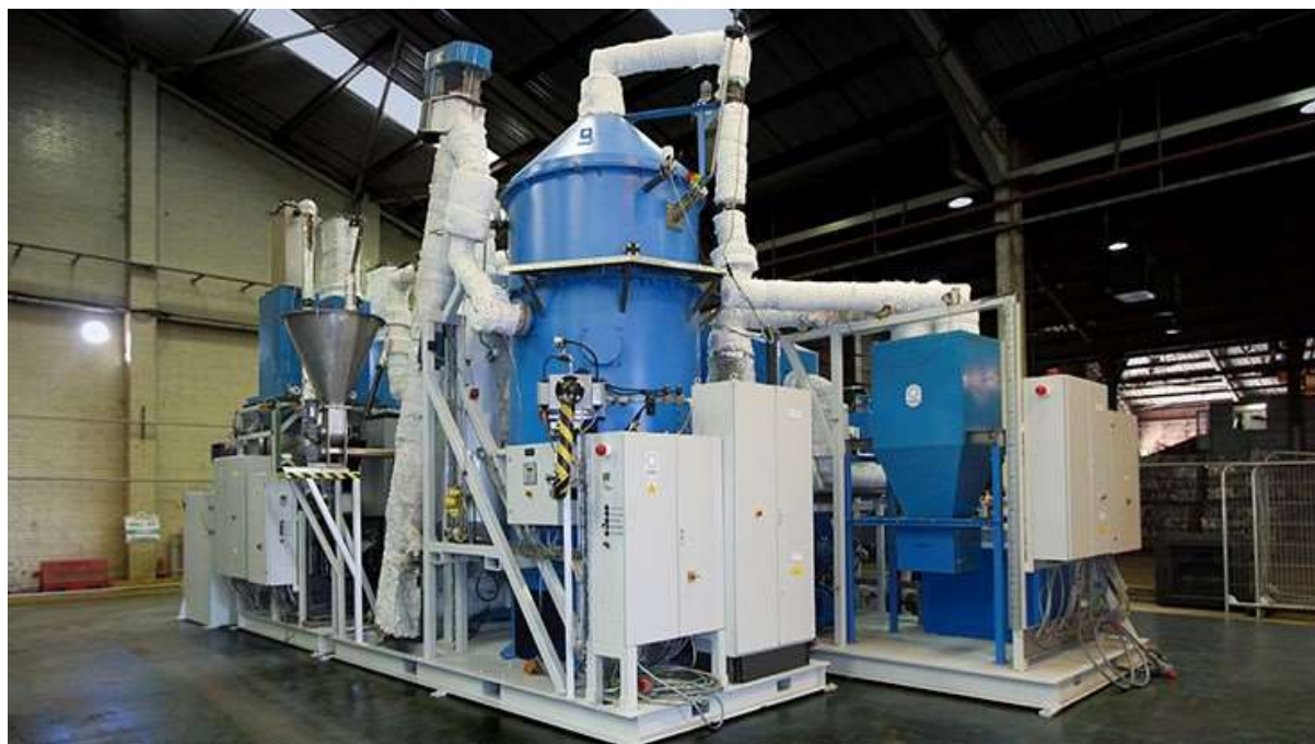
Figure 3-9: The Plaxx RT7000 processor for converting mixed plastics into fuel (source: Recycling Today, 2017)
