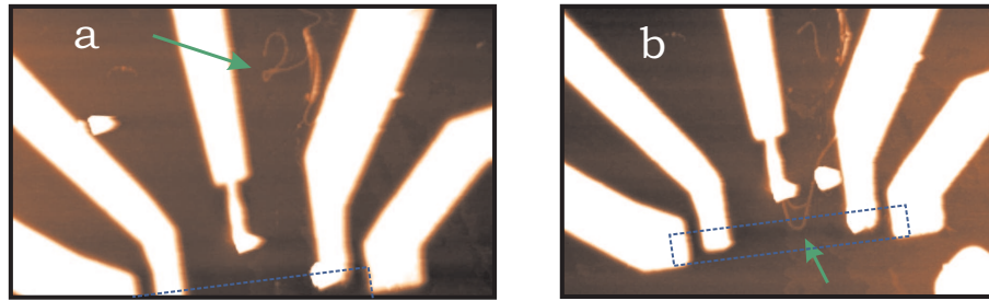
Figure 5.9: MWCN manipulation on a graphene sample. Initial (a) and final (b) positions of the nanotube (highlighted with the green arrow) imaged with TAFM.
